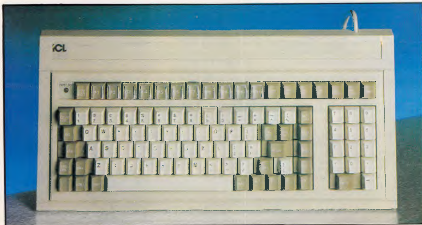
The keyboard is well pitched and has 102 keys of various shapes, sizes and colours
